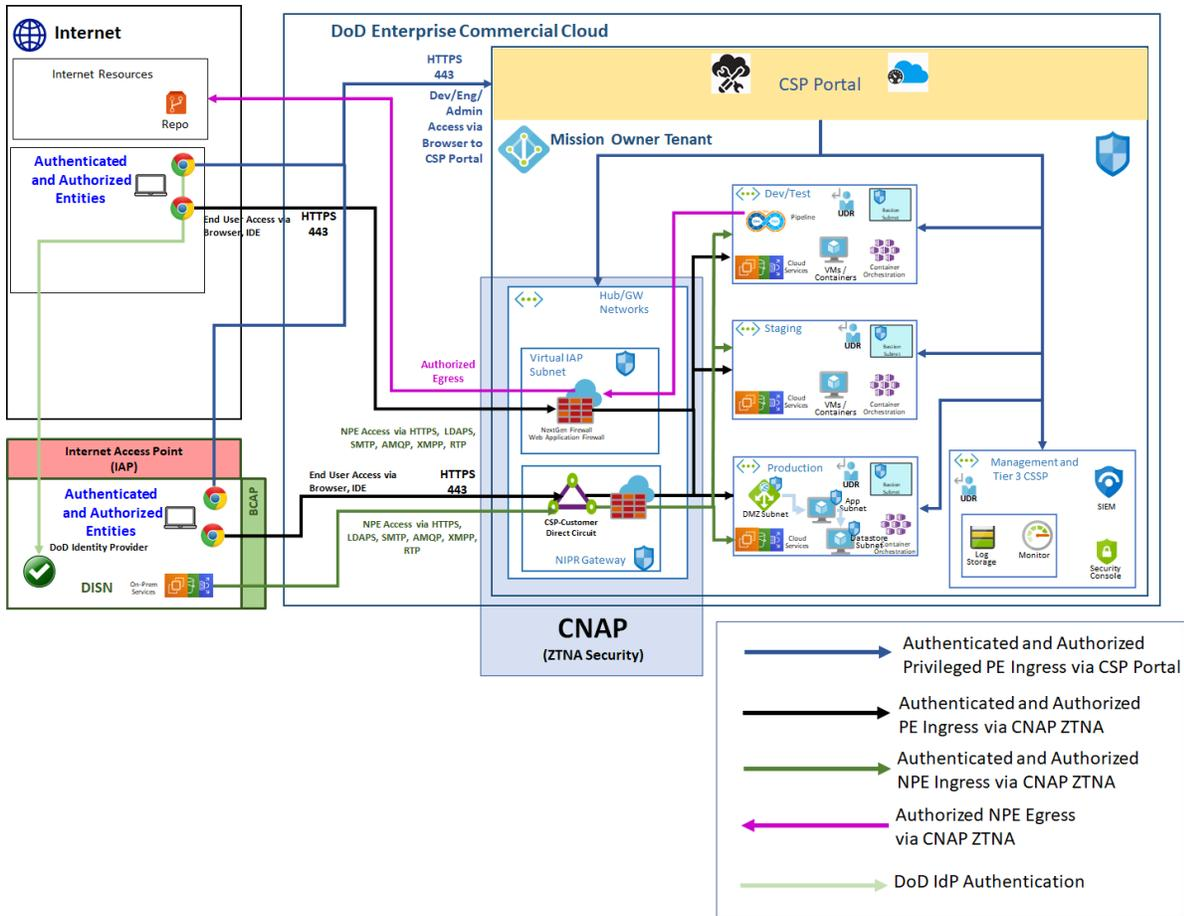
Figure 6 – CNAP Access to MO Enclave
